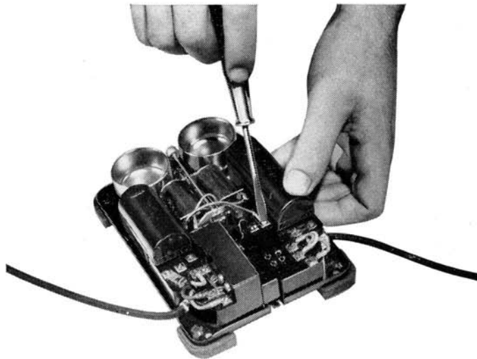
Figure 24 — Reversing Ringer Leads
