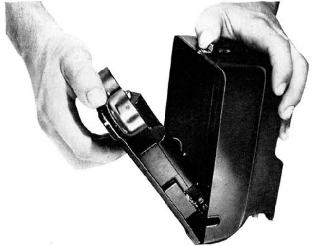
Figure 10 — Removing Wall Housing
