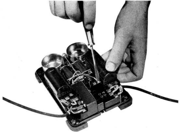
Figure 13 — Reversing Ringer Leads
