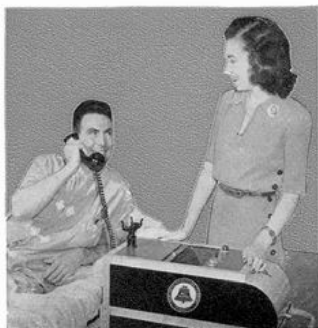
"Telecart," a miniature switchboard on wheels, invented by Company engineers, enables hospitalized Service men to make calls.
