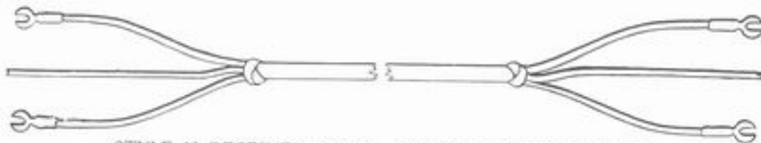
STYLE H RECEIVER CORD. SPADE CLIPS BOTH ENDS.
