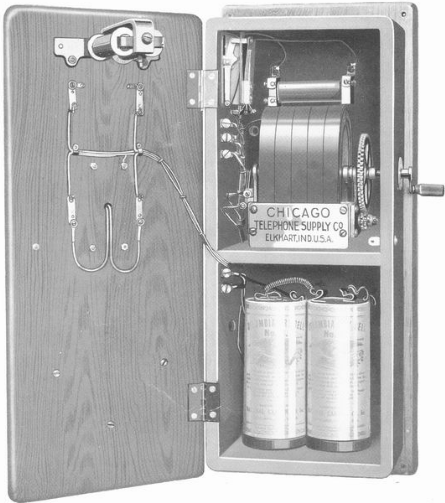
CHICAGO DE LUXE TELEPHONE OPEN CABINET
