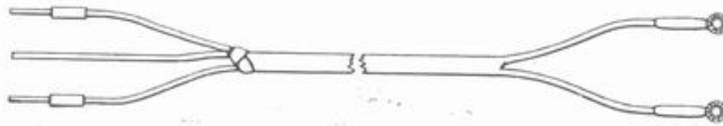
STYLE C RECEIVER CORD. SOLID TIPS ONE END. LOOPS OTHER END.
