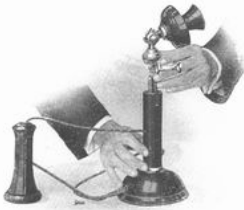
FIG. 3—LIFTING INTERIOR ASSEMBLY COMPLETE FROM SHAFT OF STAND
