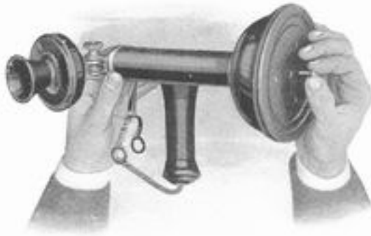
FIG. 1—REMOVING MASTER-SCREW FROM BASE OF STAND
