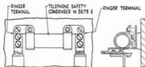
Safety Condenser fixed on N2961.
