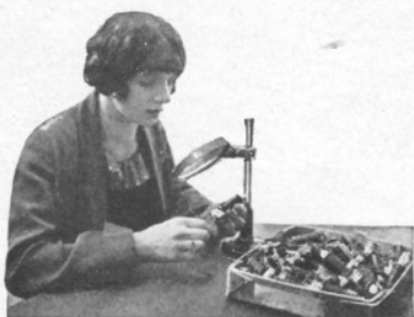
Copper wire wrapped with cotton and silk around iron cores makes the relay coils this girl inspects.
