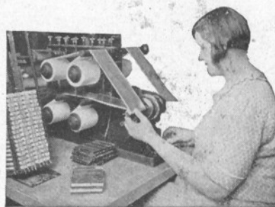
Condensers used in telephone circuits are made by rolling together alternate sheets of foil, made from tin and antimony, and thin paper. The finished condensers are enclosed in metal cases. (Some condensers are made by stacking alternate layers of mica and tin foil.)
