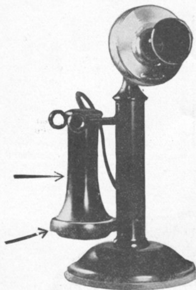
Sheet rubber baked and vulcanized is used for the receiver of your telephone and moulded rubber dust is used to form the cap of the receiver.
