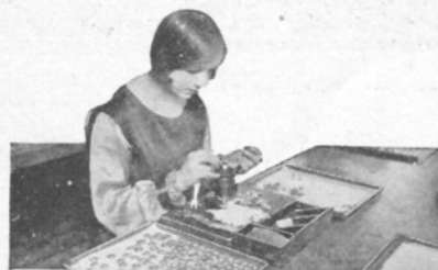
A round piece of mica forms one end of the carbon transmitter button of your telephone instrument.
