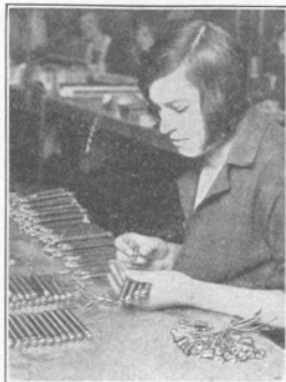
There is lead in the telephone fuse wires which protect the telephone circuits.
