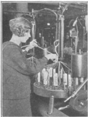
Cotton braid protects many types of telephone cords. As the insulated wires or cords come up through the center of this machine, spindles of cotton thread move in and out and round and round braiding on the protective layers.
