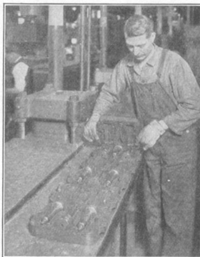
To make a telephone receiver, a sheet of rubber, shaped to form half a receiver, is laid in a mould then a metal core is laid upon it and another sheet of rubber is laid over the core. Thereupon the operator puts the top on the mould and it is ready to be loaded on the truck and sent away to be baked.
