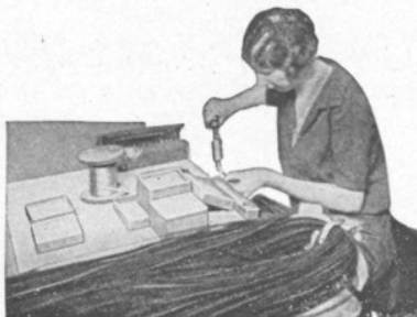
Pure silk covers the cords and wires of your telephone. Silk is strong, flexible and is a good insulator.
