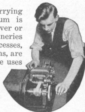
The combination of gold, silver and platinum resists corrosion and wear. From thin ribbon such as this man is making, discs are punched and welded onto springs to provide contacts.
