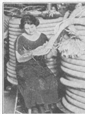
This shows the paper wrapped wires in a cable and the paper wrapping around the entire rope-like group of wires, just as the cable core looks before it receives its sheath of lead and becomes real lead covered cable.
