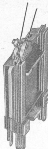
There are contact points of gold, silver and platinum between the leaves of this relay and when a current passes through and operates it, making some of the leaves go together, the contact points establish new pathways for currents and thus the relay performs its part in a telephone conversation.
