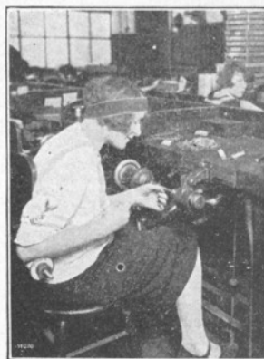
Insulated thin copper wire is wound around iron rods in your telephone receiver to make a magnet.
