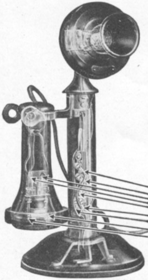
Solder, a lead and tin alloy, joins connectors to the telephone cord wires and receiver coil terminals.
