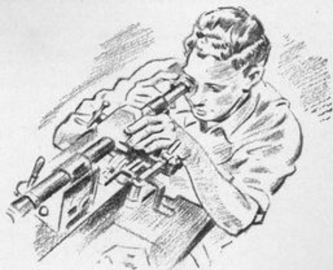
Quartz crystals cut accurately to within \frac{1}{25,000} of an inch.
