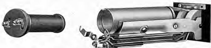
Fig. 5—Coil Removed and Leads Disconnected
