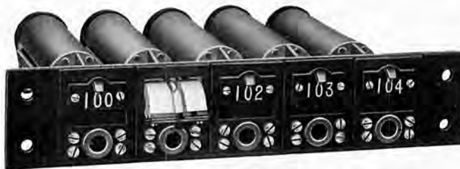
Fig. 3—Front View, Bank of No. 11 Drops
