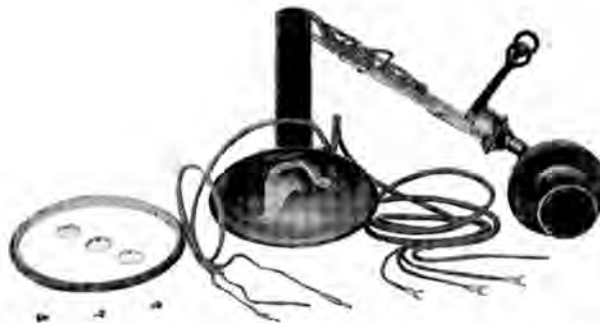
By removing the screws in the base plate, the Desk Stand may be resolved into its three principal parts, as shown above
