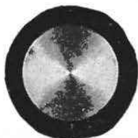
Enlarged Cross Section of Copper Clad Wire
