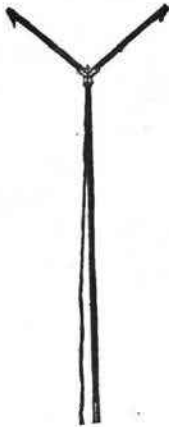
End Section with Spreaders Extended No. 3 Line Pole
