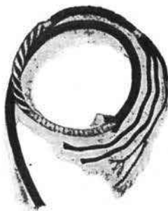
Construction of Moisture-proofed Tinsel Telephone Cords
