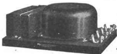
No. 1A Repeating Coil Group
