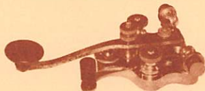
The No. 1 Lewis Legless Telegraph Key, Western Electric Manufacturing Co. catalogue 1878, $5.00.
